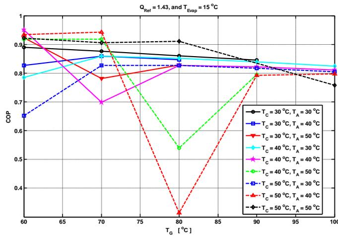
**Figure 9: The Relationship between the Coefficient of Performance and Heat Generator, at  $T_e=15^\circ\text{C}$**
