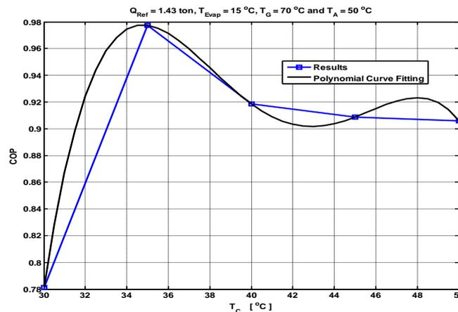
Figure 12: The Relationship between the Coefficient of Performance and the Condenser Temperature, When Generator Temperature Equal  $70^\circ\text{C}$ , and Absorption Temperature Equal  $50^\circ\text{C}$
